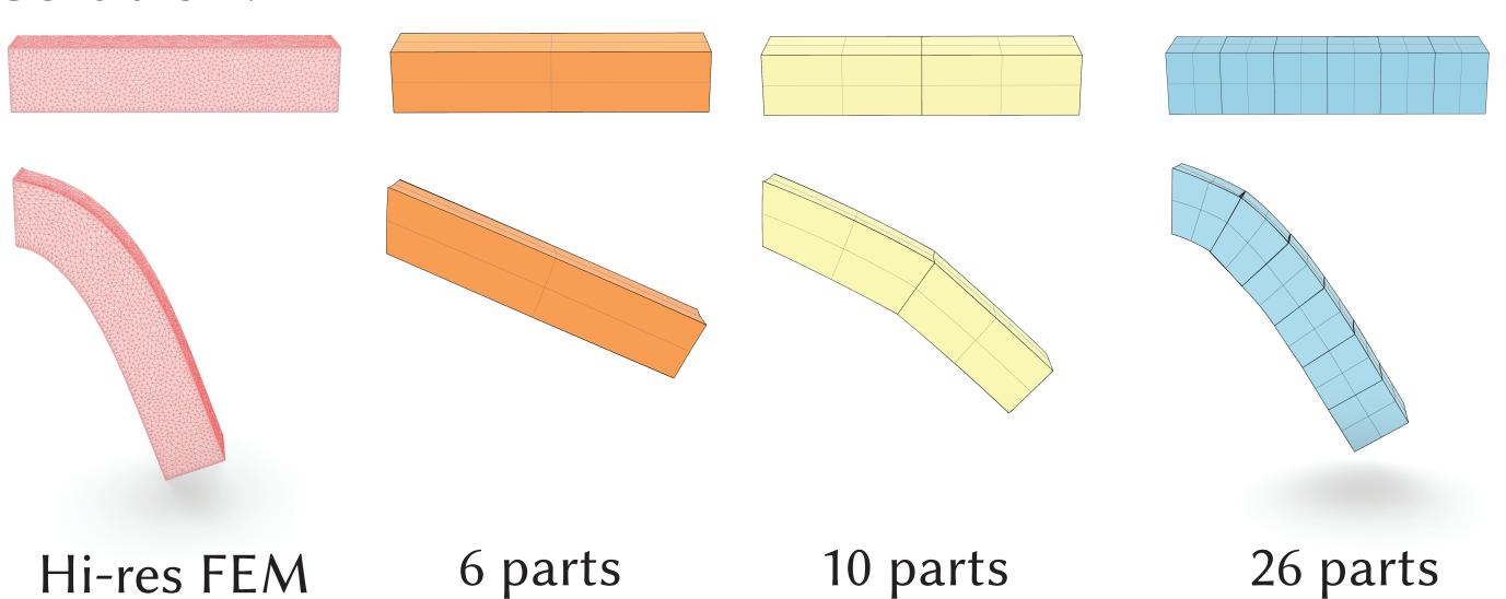
Handles Large Deformation With relatively few NURBS parts, we can simulation this beam twisting with no instabilities.
