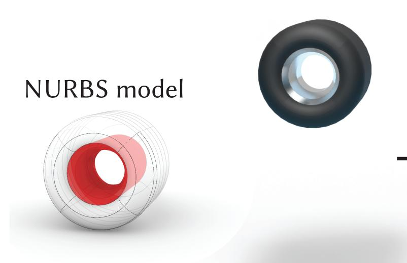
**Directly Editable Output** SEM simulates on the original NURBS degrees of freedom, so the output is digestible by the same software used to design the model.
