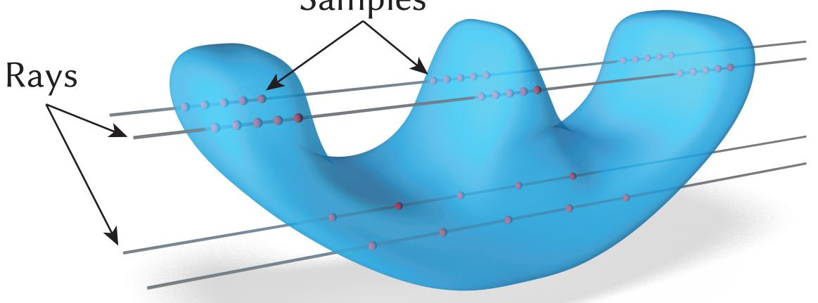
**Blending Weights** Meshless construction by raycasting
